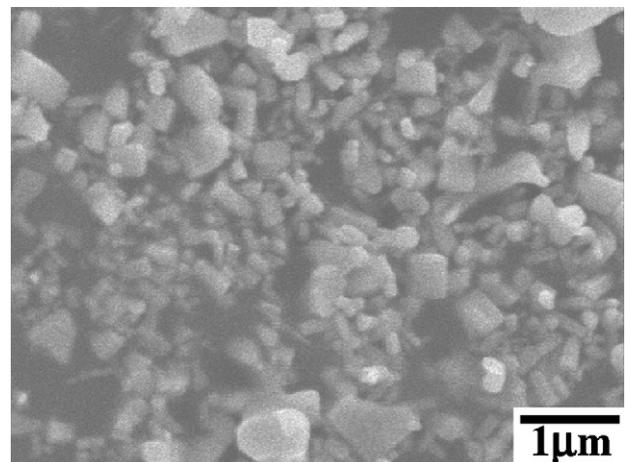
Fig. 3. SEM photograph of ZnO particles.
