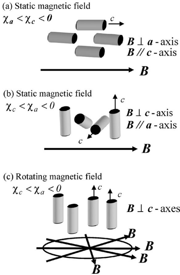
Fig. 1. Schematic illustration of a particle in a slurry in a static or a rotating magnetic field. (a) static magnetic field,  $\chi_a < \chi_c < 0$ , (b) static magnetic field,  $\chi_c < \chi_a < 0$ , (c) rotating magnetic field,  $\chi_c < \chi_a < 0$ .
