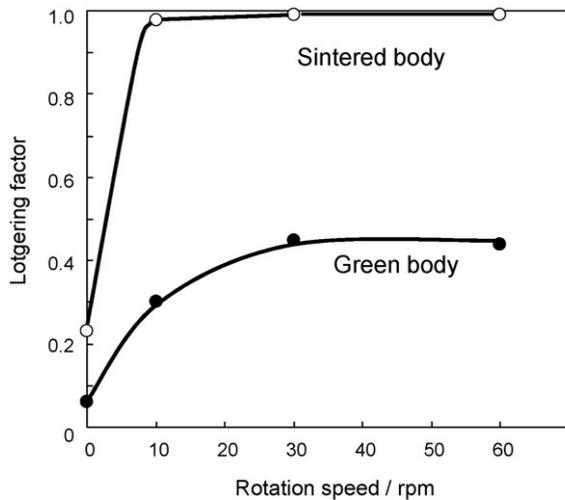
Fig. 7. The influence of rotation speed on Lotgering factor of green and sintered body.
