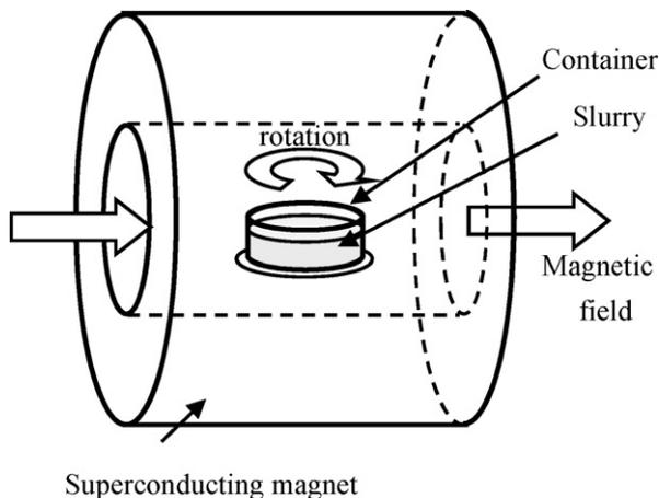
Fig. 2. Schematic illustration of rotating a container containing slurry in a static magnetic field.
