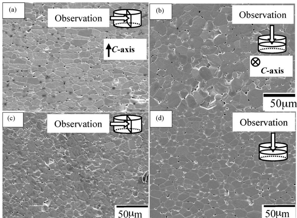
Fig. 6. The microstructure of the sintered ZnO ceramics observed from the directions parallel (a) and perpendicular (b) to the axis of the rotating magnetic field. The microstructure of ZnO formed without magnetic field, (c and d) microstructure observed from the same directions with (a and b), respectively.
