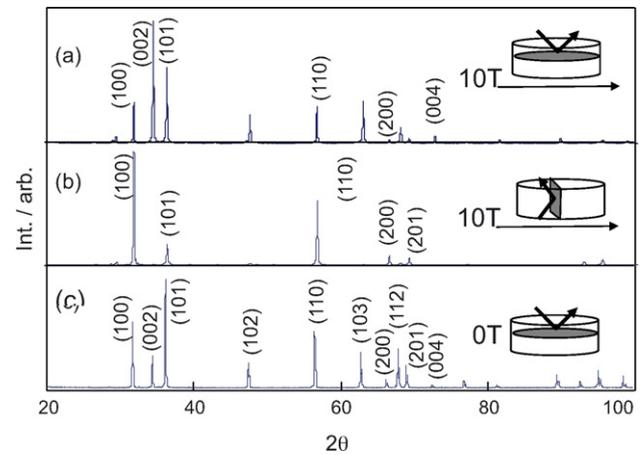
Fig. 5. XRD patterns of sintered ZnO formed with a static magnetic field, (a) the plane in the direction parallel to the magnetic field, (b) the plane in the direction normal to the magnetic field, (c) no magnetic field.<sup>19</sup>
