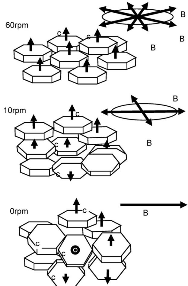
Fig. 8. Schematic estimated illustration of the oriented ZnO crystallites prepared in rotating magnetic fields (from 0 to 60 rpm).
