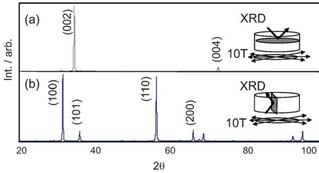
Fig. 4. XRD patterns of sintered ZnO formed by a rotating magnetic field, (a) the plane in the direction parallel to the rotating magnetic field, (b) the plane in the direction normal to the rotating magnetic field.<sup>19</sup>
